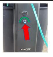
**OPERATING YOUR O₂REMOTE**: push the power switch to turn on power. Push either "IN" or "OUT" on the remote to operate. Turn speed dial to adjust speed.
